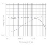
The nano-composite frequency response is much more consistent than a diaphragm composed of traditional materials. ......Silica/PA66 Nano-composite Sheet (QUALIA 010) --- PET Film (traditional materials) — Sony MDR-M10 Headphones
